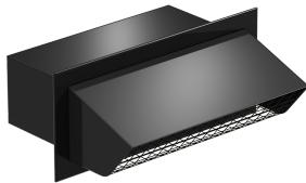
Hooded wall cap with rectangular duct connection designed for outside wall applications. Constructed of steel with black enamel finish, units feature built-in birdscreen and damper.
