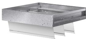
The WD-410 series are non-motorized backdraft dampers which may be mounted either vertically for intake air or mounted horizontally to allow vertical airflow down and prevent reverse airflow. The dampers are opened by air pressure differential and closed by springs.
