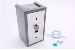
NEMA-1 rated disconnect switch provides positive electrical shutoff and safety. Disconnect switches are a recommended and necessary safety feature for every fan. Mounted directly on the fan, within sight and reach, disconnect switches provide the best protection against accidental startup during service or inspection.
